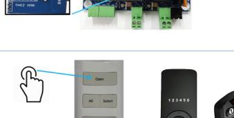
Step 3: While on CH 1, Press "Open" (or up on the slimline) on the new remote.
