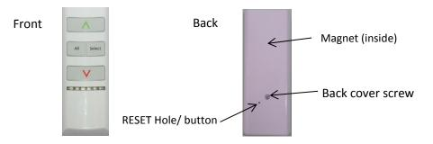
**Battery Replacement** On the back of the remote control remove the screw using a small Phillips screwdriver. Loosen the back by inserting the flat screw drive between the seams on both sides, top, middle and bottom. Gently remove the back cover. Replace the battery with a **GP23A** 12V battery.
