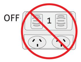
2. Isolate power point 1 by cutting the power from he mains (or disconnecting from the wall).
