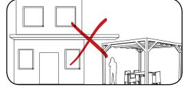
DO NOT install under roof lines or eves.
